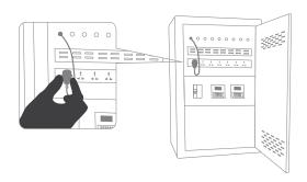
Please open the back door, then connect laptops charging interface and plug on the outlets.
